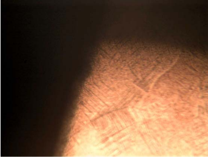
Figure 4-25 Microstructure of conventional speed machined specimen# 6 at 120x magnification showing the orientation of the grains
