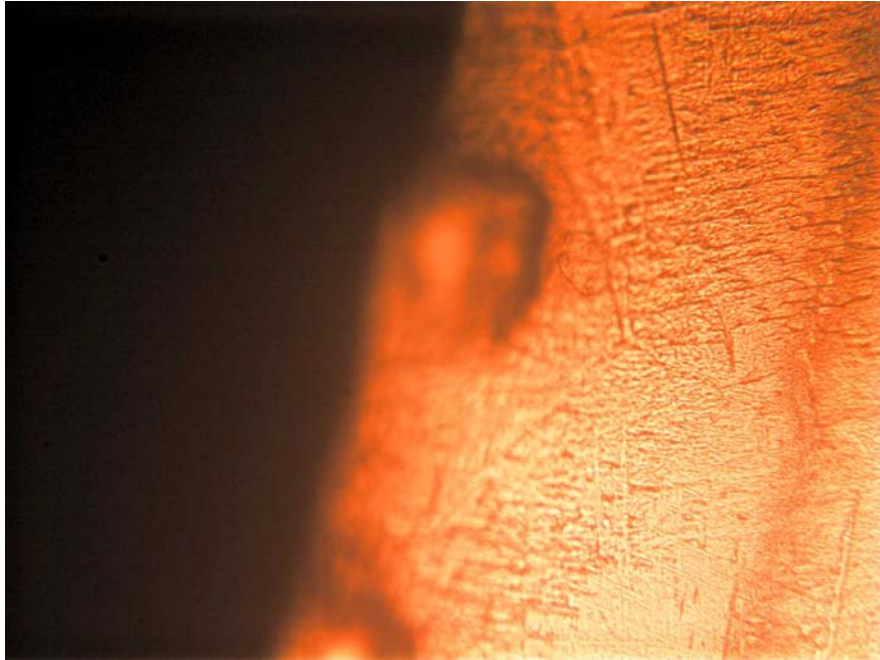
Figure 4-27 Microstructure of high speed machined etched specimen# 6 at 250x showing the surface defects at location #1
