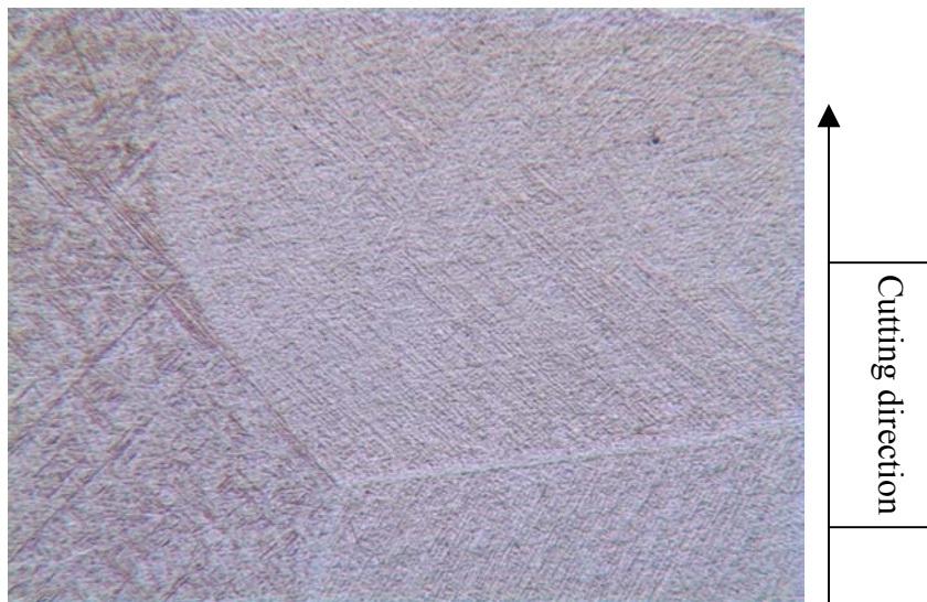
Figure 4-13 Microstructure of conventional machined process specimen #2 at magnification 120x
