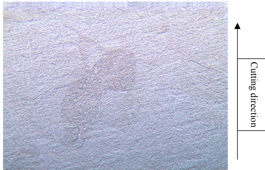
Figure 4-14 Microstructure of advanced machined process specimen #7 at 40x
