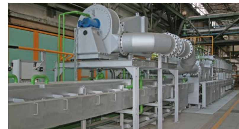
Bright annealing furnace at the mill in Costa Volpino, Italy
