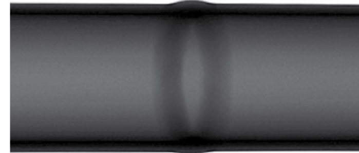
Umbilical joint inspected by x-ray system
