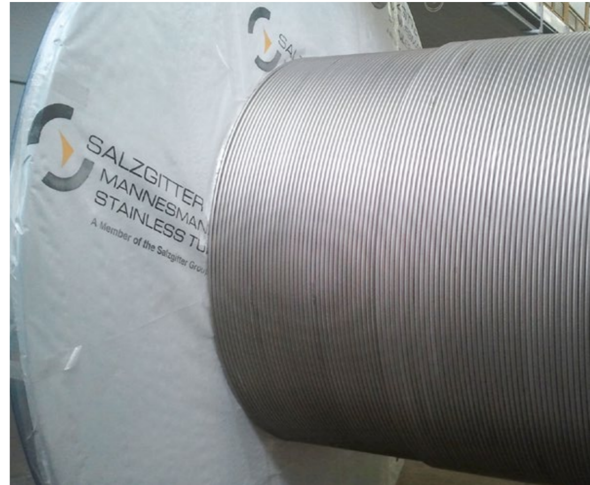
Reeling system at umbilical line
