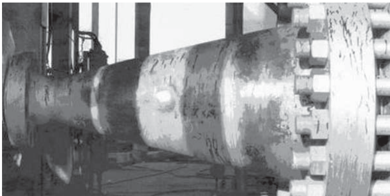
8.21 The conical inlet that suffered damage.
