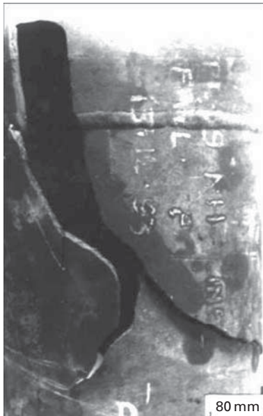
8.1 The failed condenser tube.
