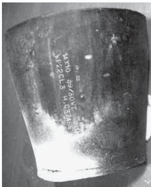
8.5 The failed steam reducer.
