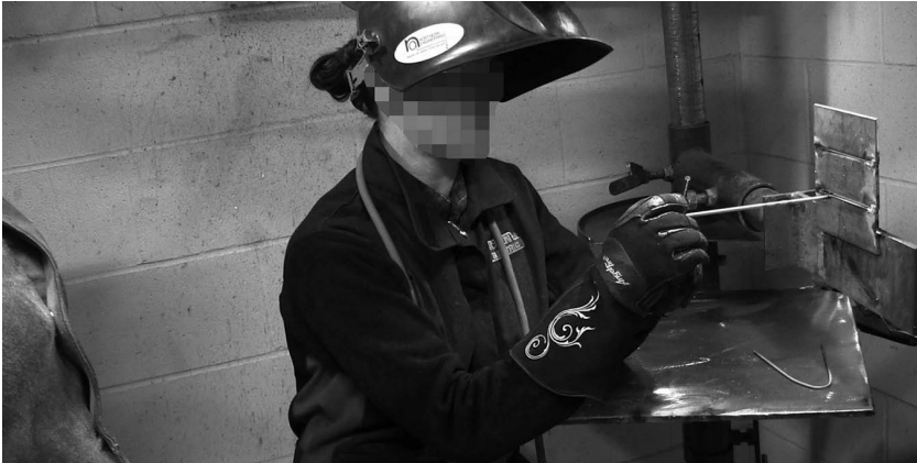
Figure I.26. Teresa demonstrated the dig-and-fill method as she described her movement: “Coming back and pushing it in.” Then, she gestured, using the electrode as a pointer.
