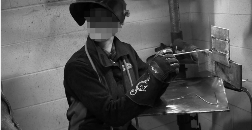
Figure 3.11. Teresa demonstrated the unwanted action of pulling the electrode out of the weld joint as she directed, “You don’t want to pull it out of the plates.”
