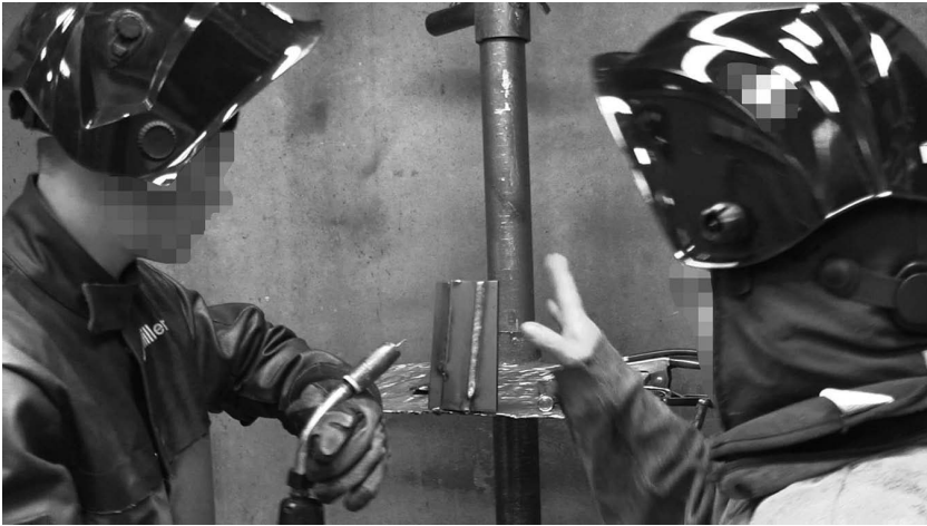
Figure 4.4. Tonya asked Steve a pumping question that pushed Steve to interpret the meaning of the physical characteristics of the weld that he had just produced: “See how the puddle’s getting ahead of you?”
