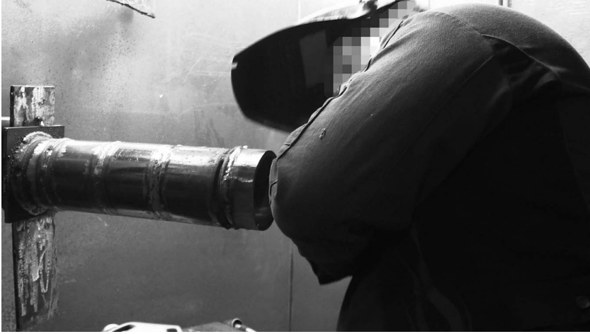
Figure 3.5. Tom began demonstrating body position for welding around a pipe while using a phonetic metaphor: “And it’s just a roooll around the pipe.”
