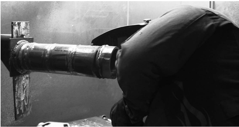
Figure 3.6. Tom finished demonstrating body position for welding around a pipe while using a phonetic metaphor: “And it’s just a roooll around the pipe.”
