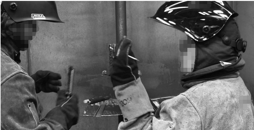
Figure 3.13. Tonya demonstrated the difference between an effective and an ineffective travel angle with an electrode. She started the demonstration with the electrode pointed slightly up.
