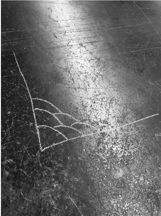
Figure 1.2. Soapstone drawing of a multipass weld on a metal table.
