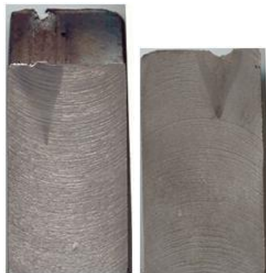
Figure 41. The heat affected zone geometry at beam current 100 mA, welding speed 0.5 cm/s and the distance to the sample surface: a) 238 mm in surface 3 (Figure 40); b) 352 mm at surface 1a (Figure 40)]
