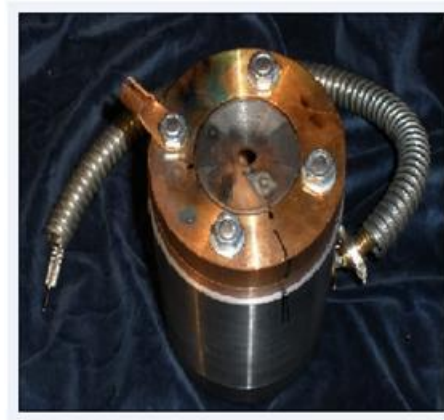
Figure 28. Photography of the set for measuring radial current distribution of EBW beam utilizing the method of Dr. Elmer. The tungsten sampling disc have 7 radial slits
