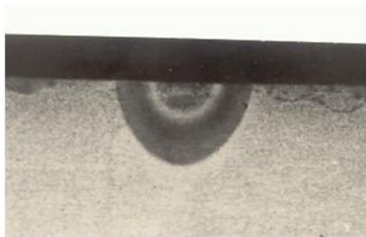
Figure 30. Weld cross-section at EB power density less than 106 W/cm 2
