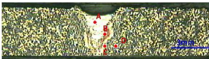
Figure 8. Macro-structure of the laser welded joint with 0.3 mm thick Ti filler
