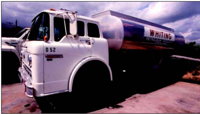
Figure 1.13—Aluminum’s Light Weight and Corrosion Resistance is Very Suitable for the Fabrication of Many Types of Tanker Trucks
