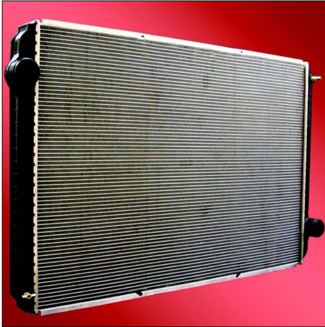
Figure 7.17—A Controlled Atmosphere Brazed (CAB) Aluminum Radiator Core with Mechanically Attached Nylon Tanks. This Heat Exchanger is Used on a Class 8 Truck.
