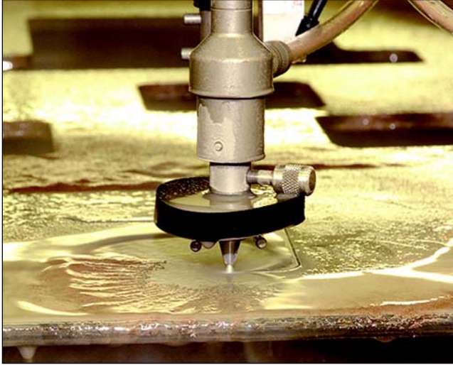
Figure 6.35—Extremely High Quality Precision Cutting of Aluminum with Abrasive Water Jet
