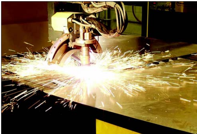
Figure 6.33—High Speed Conventional Plasma Arc Cutting of Aluminum Sheet
