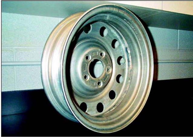
Figure 1.1—Fabricated Wheel Often Manufactured from the 5xxx Series Aluminum Base Alloys
