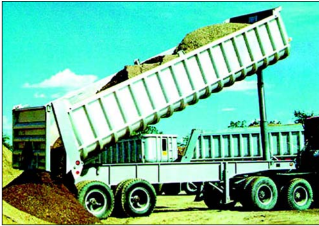
Figure 1.10—Dump Trailer Usually Built from 5xxx Series and 6xxx Series Aluminum Alloys
