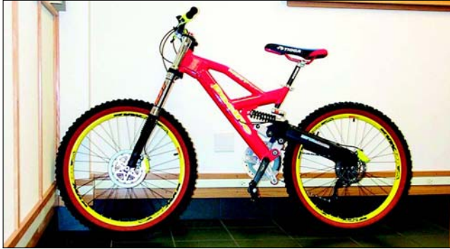
Figure 1.7—High-Performance Bicycle Made from 7xxx Series Aluminum Alloy
