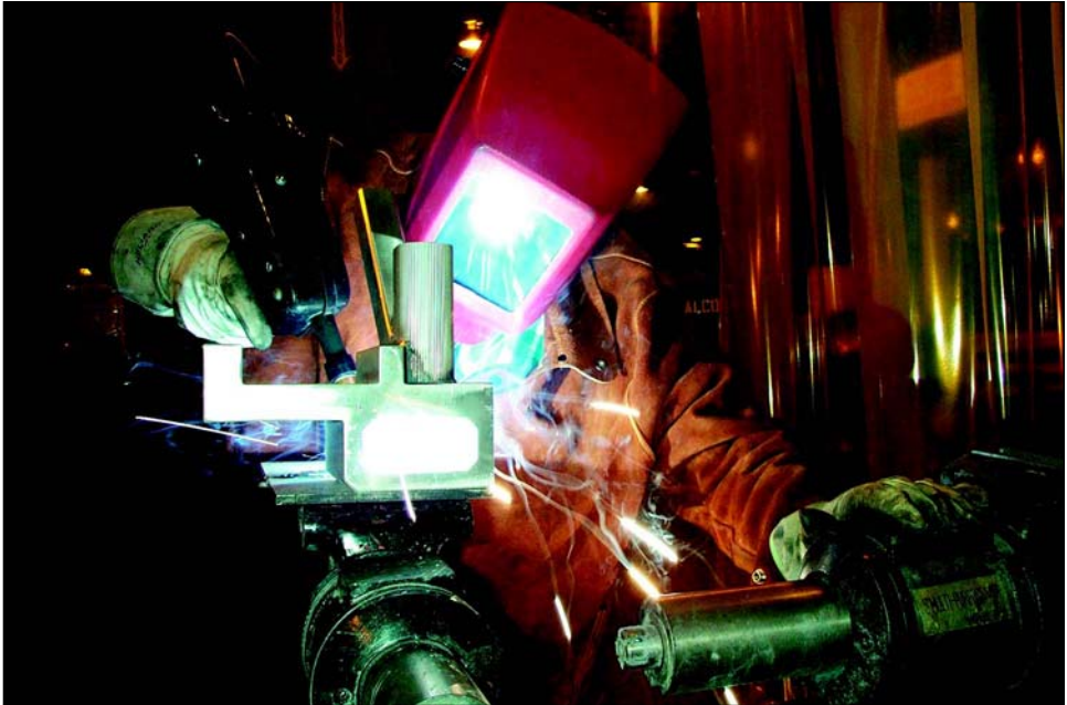
Figure 6.1—GMAW Welding an Aluminum Extrusion Using a Spool Gun
