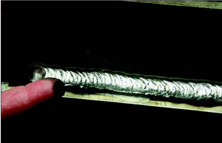
Figure 6.12—GMAW Weld with Smut—Smut Can be Removed Quite Easily by Wiping Soon After Welding
