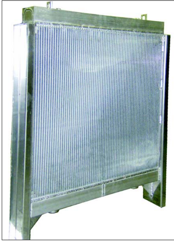
Figure 7.19—A High Pressure Oil Cooler Consisting of a Controlled Atmosphere Brazed (CAB) Brazed Aluminum Core with Extruded Aluminum Tanks that are GTAW (TIG) Welded to the Core. This is a Two Pass Oil to Air Heat Exchanger Which Operates at 500 psi.
