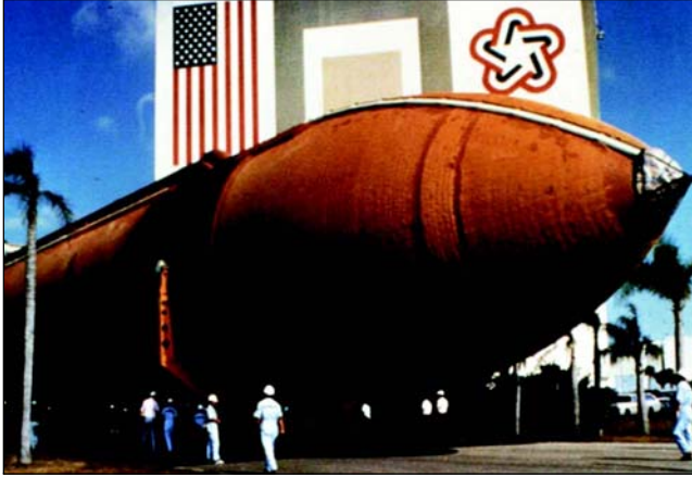
Figure 1.17—The Space Shuttle Fuel Tank is Fabricated from High-Strength Aluminum Alloys
