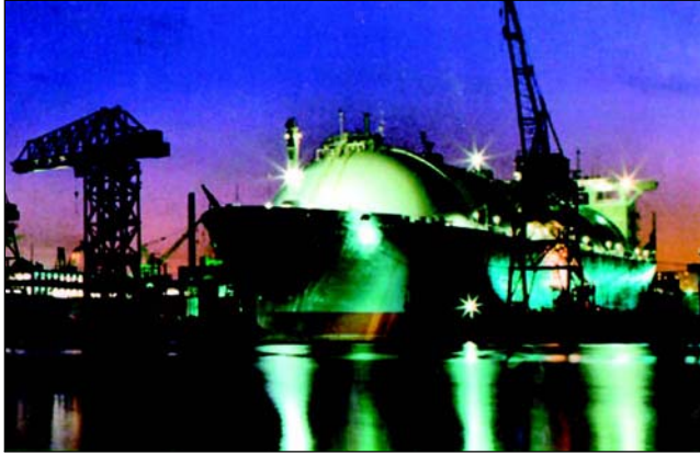
Figure 1.12—LNG Tankers Make Use of the Low-Temperature Strength of Aluminum Used for the Manufacturing of These Large Spherical Vessels
