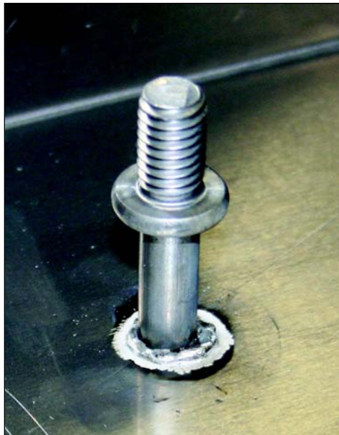
Figure 6.30—Aluminum Fastener Stud Welded to Aluminum Plate
