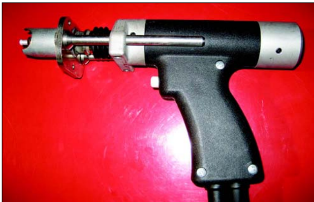
Figure 6.32—Hand Held Gun for Capacitor Discharge (CD) Stud Welding
