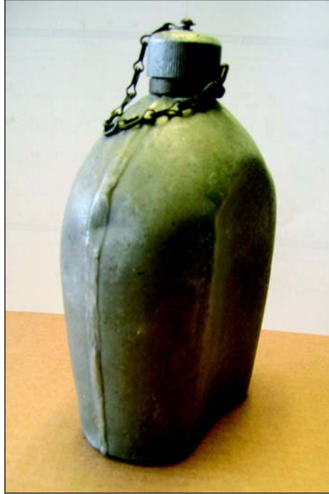
Figure 2.2—U.S. Military Water Bottle Stamped 1918 and Welded with the Oxyfuel Gas Welding Process
