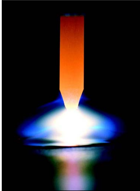
Figure 6.7—Open Root Joint Welding of Aluminum Pipe is Predominantly Performed by the GTAW Process, Using AC Current to Produce an Arc Between a Tungsten Electrode and the Aluminum Plate and Protecting the Molten Aluminum with Pure Argon Shielded Gas
