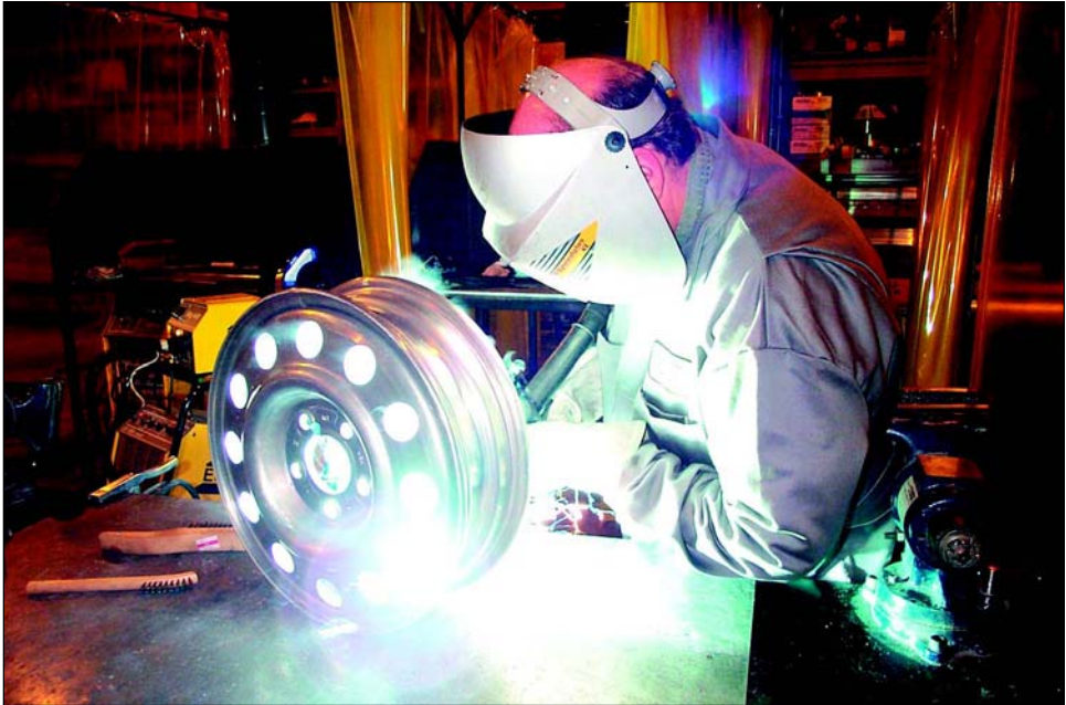
Figure 4.1—Gas Metal Arc Welding on an Aluminum Wheel Uses 5454 Base Material Welded with an ER5554 Filler Alloy that is Made Specifically to Match the Base Alloy Content
