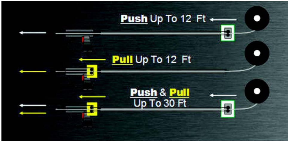
Figure 7.13—The Different Types of Feeding Systems for Aluminum Welding
