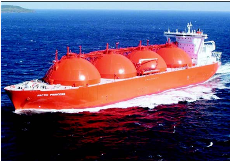
Figure 3.14—Liquid Natural Gas (LNG) Tanker with Four Large Welded Aluminum Spheres (Tanks)
