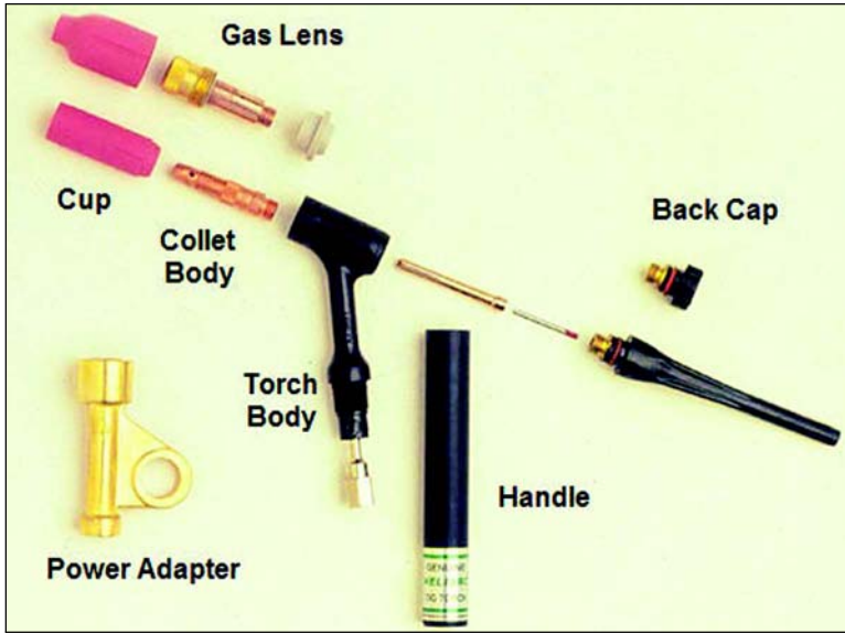
Figure 7.5—GTAW Torch Components
