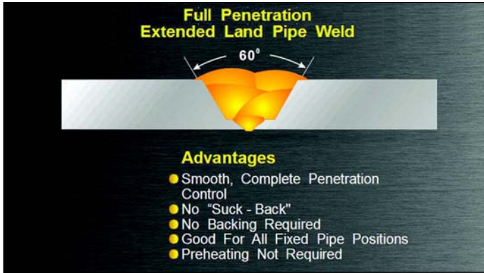
Figure 6.8—Extended Land Pipe Weld with the Advantages Listed for This Type of Weld Preparation when Used for Aluminum Pipe Joints
