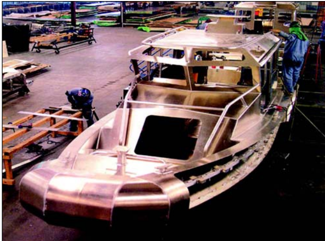
Figure 1.6—Coastguard Vessel Made from 5xxx and 6xxx Series Aluminum Alloys
