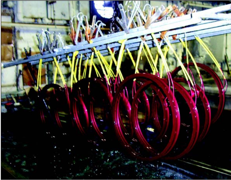
Figure 3.8—Anodized Aluminum Rings Being Removed from a Processing Tank
