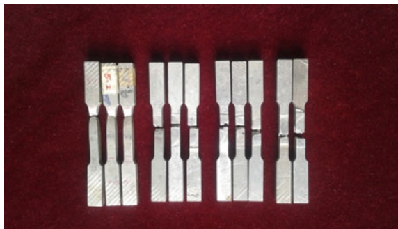
Fig. 3.10 Tensile test specimen prepared from friction stir welded AA6061/SiC/B 4 C composite [28]
