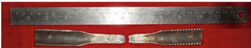
Fig. 1.30 Tensile test Specimen—fracture in weld metal
