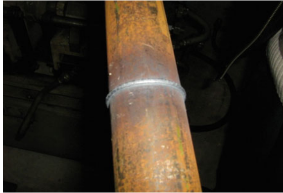
Fig. 1.22 Uniform bead and full penetration
