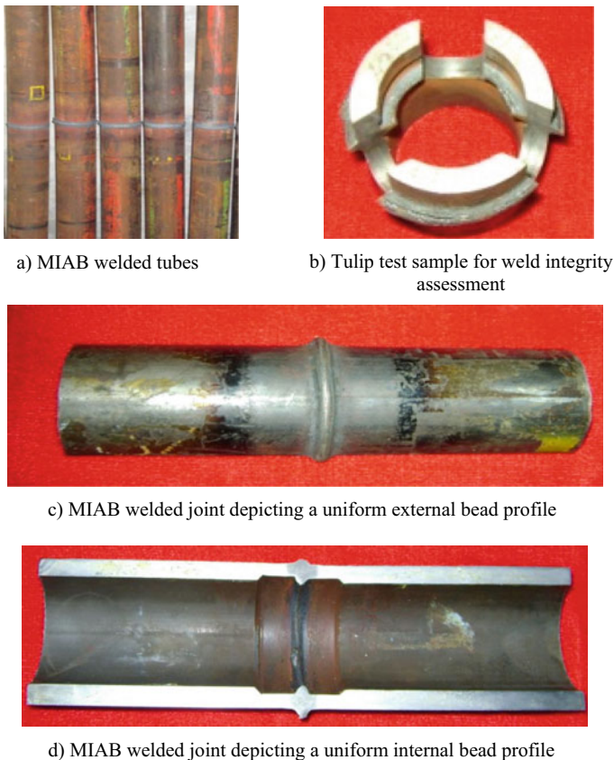
Fig. 1.21 MIAB welded joint characteristics in terms of bead profile
