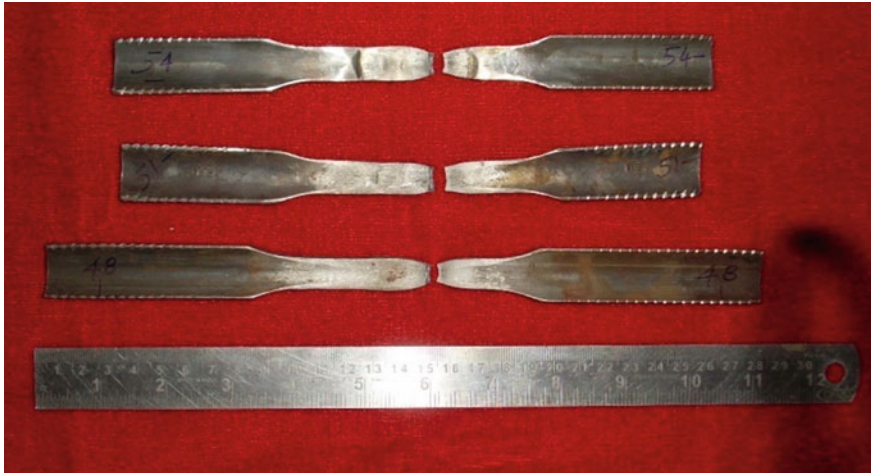
Fig. 1.29 Typical tensile tested MIAB weld tube samples
