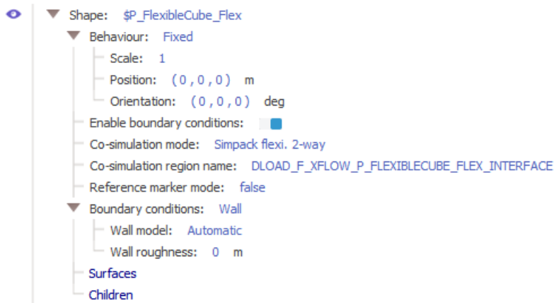
Linear flexible body import default values set in XFlow GUI
