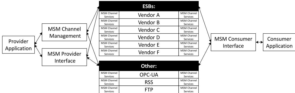
Figure 20 – Standard interface to ESBs and other message exchange systems
