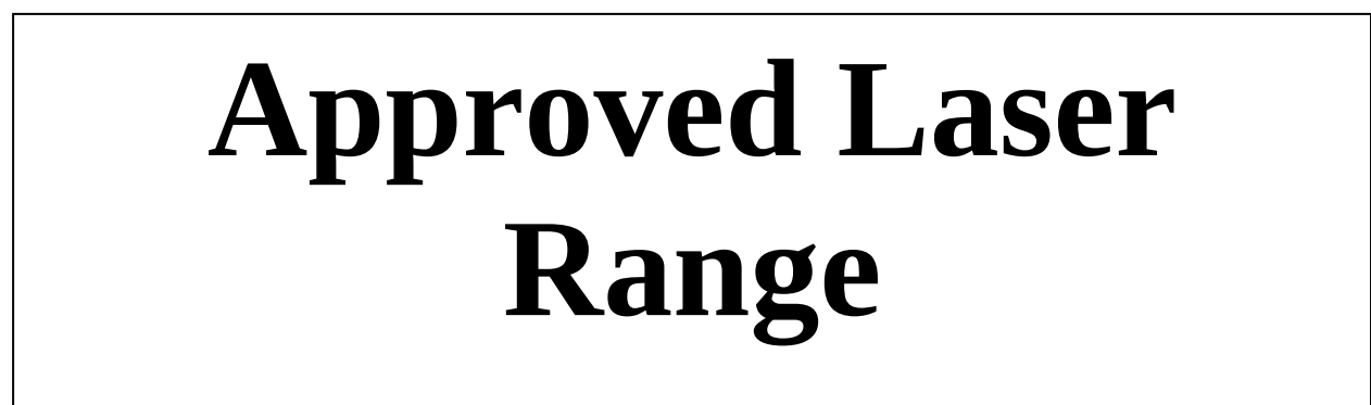
Figure 8b. Example of Permanent Laser Range Warning Sign. This sign may remain when the laser is not being used. The temporary sign would be placed in addition to this sign during actual lasing.
