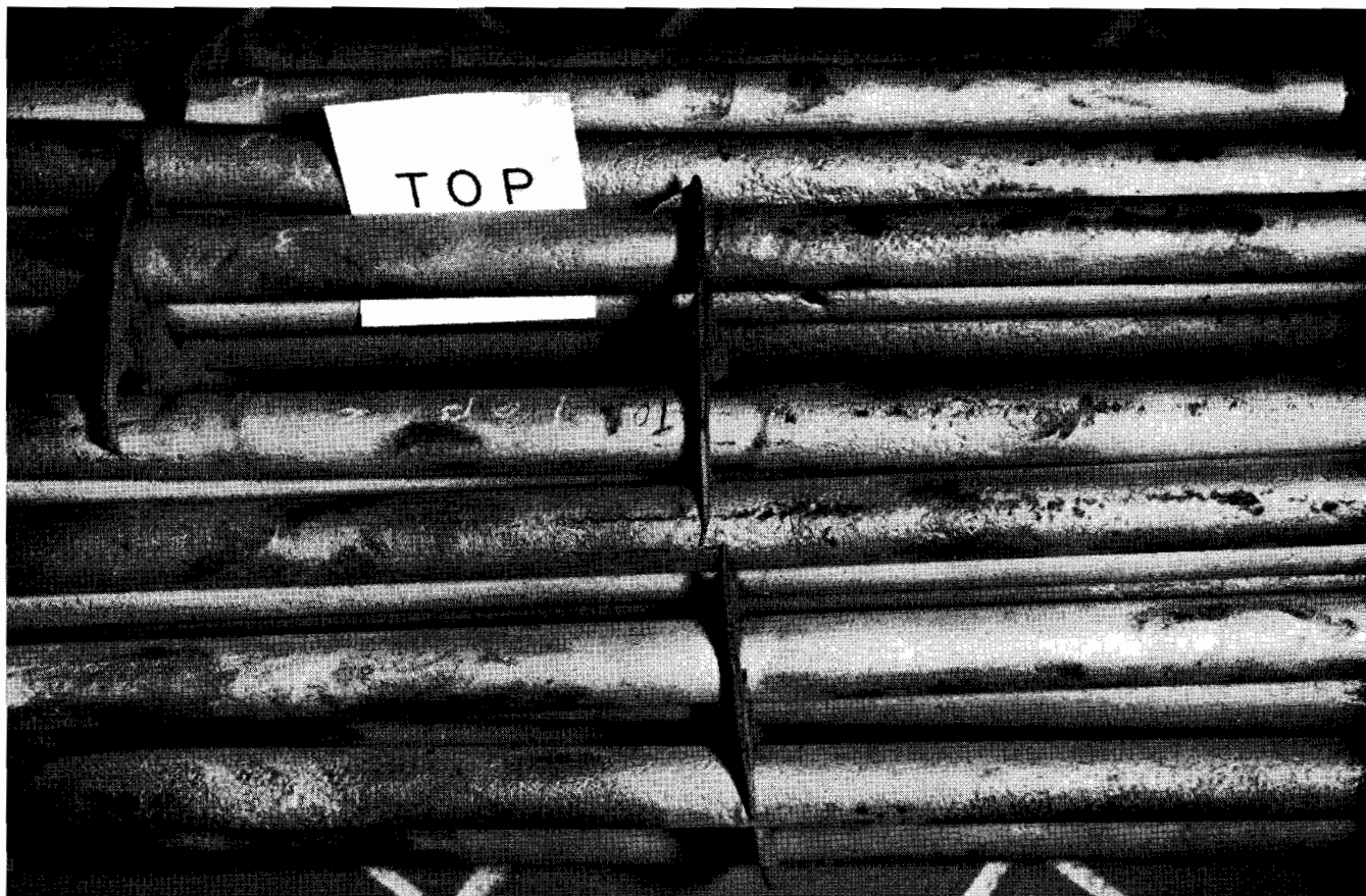
FIG. 2—Corrosion of an Admiralty Pipe Still Overhead Condenser Bundle. Most severe corrosion occurred just under the condenser inlet nozzle.
