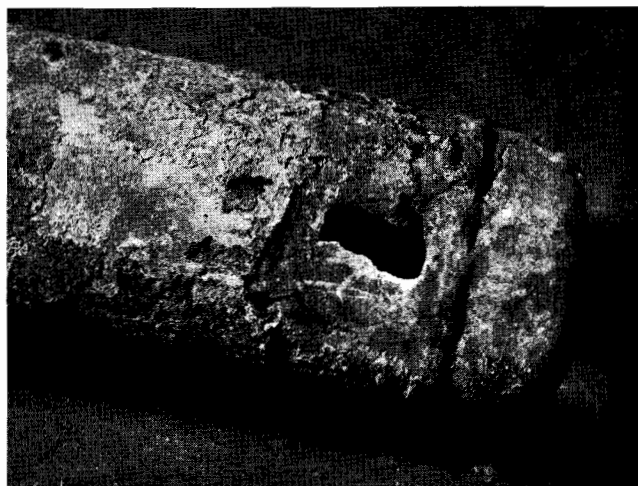
FIG. 21—Close-up of the Tube Shown in Fig. 20. Note how corrosion has concentrated near the cap and on the weld between cap and tube.
