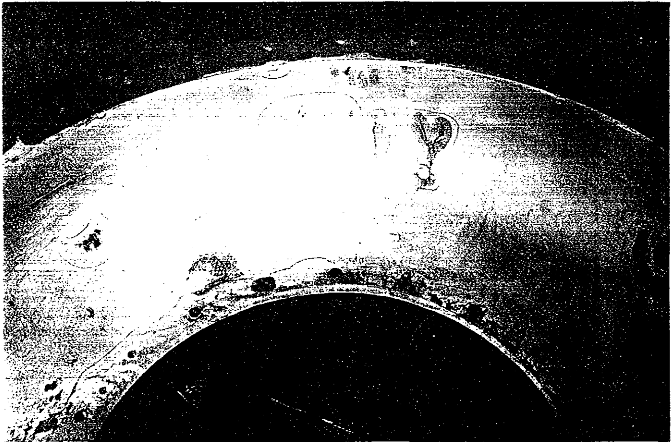
FIG. 32—Intergranular Corrosion in an 18 Chromium-8 Nickel Steel Pressure Vessel Head. Carbide precipitation occurred during fabrication. The process stream contained inorganic aluminum chloride and organic methyl and ethyl chlorides. The oil seeping out of the cracks was applied during inspection by the fluorescent-penetrant method.
