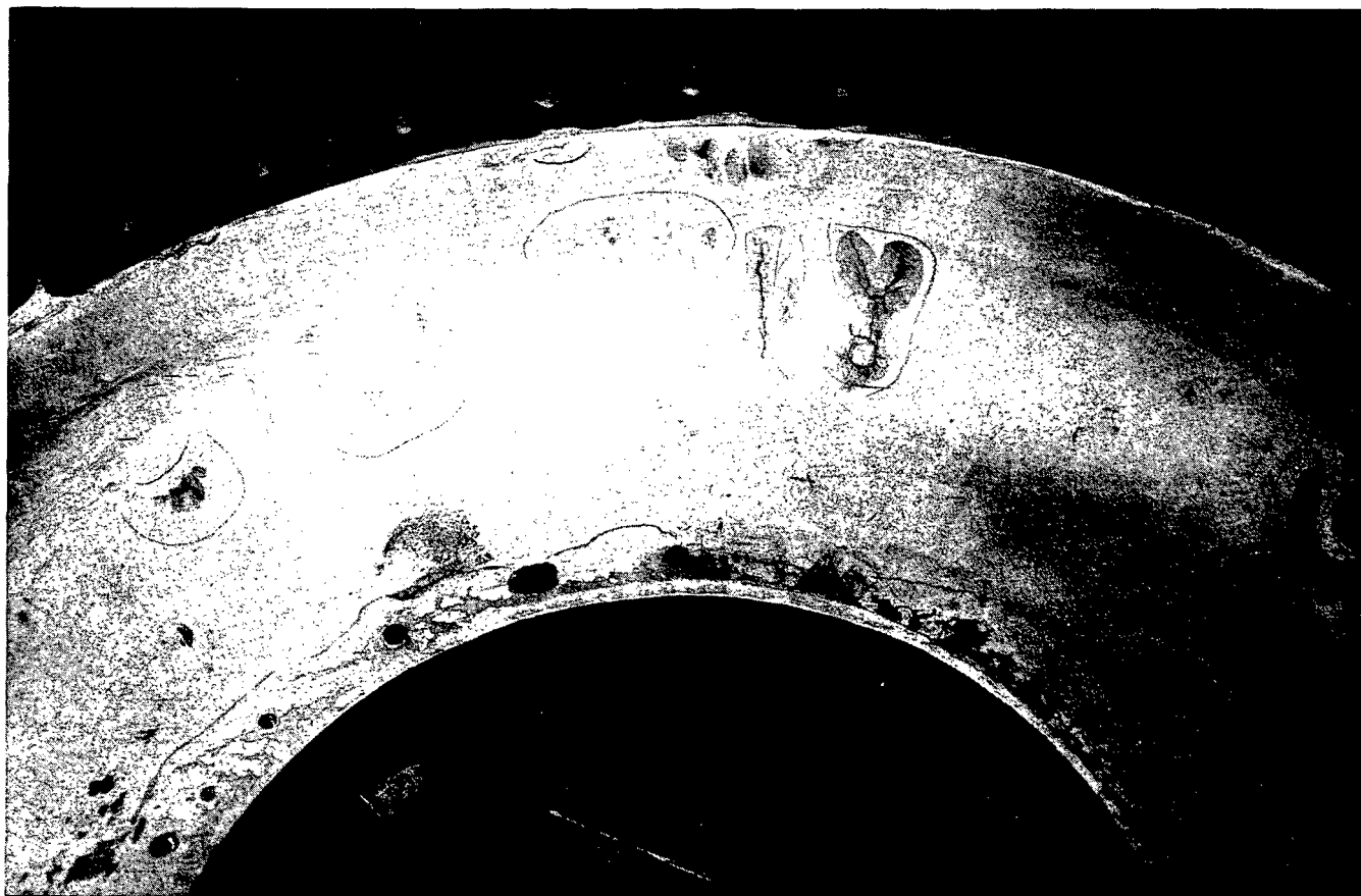
FIG. 32—Intergranular Corrosion in an 18 Chromium-8 Nickel Steel Pressure Vessel Head.
