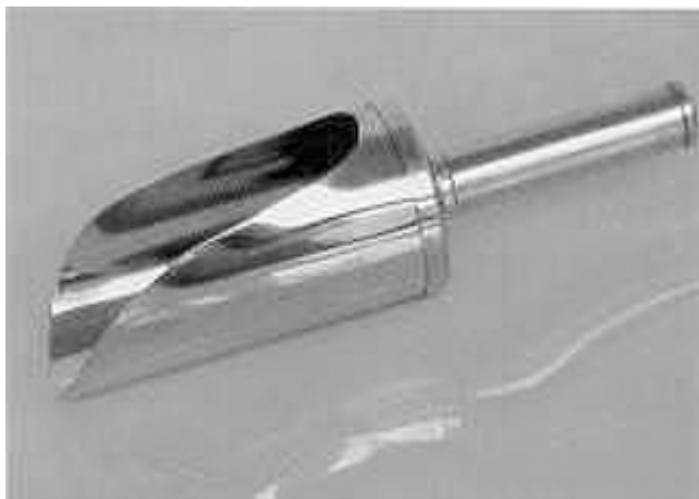
FIG. 4 Stainless Steel Scoop for Sampling Metal Powder
