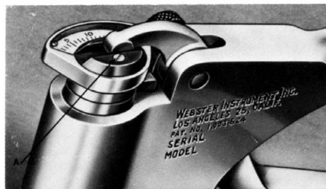
FIG. 3 Zero Adjustment Screw, A (indicated by arrow)
