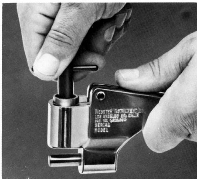
FIG. 4 Adjusting Load on Load Spring
