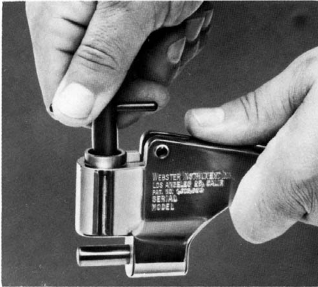
FIG. 4 Adjusting Load on Load Spring
