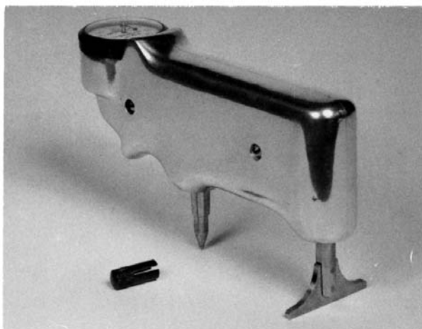
FIG. 1 Barcol Impressor, Model 934-1
