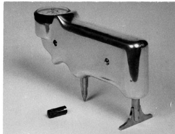
FIG. 1 Barcol Impressor, Model 934-1
