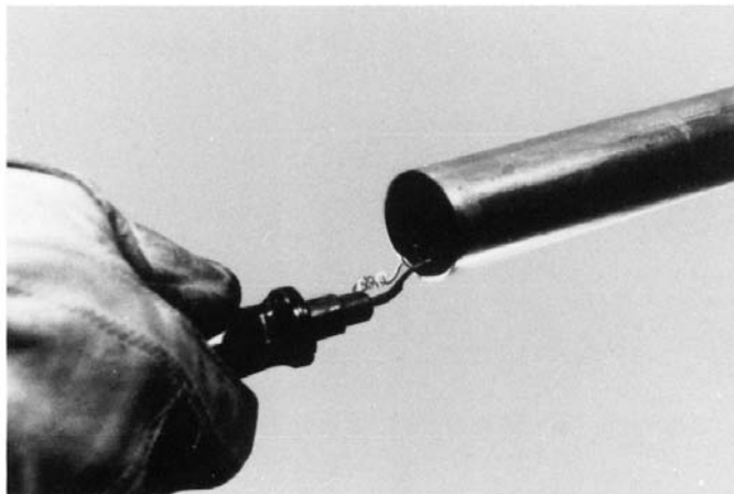
FIG. 5 Reaming: Deburring Tool
