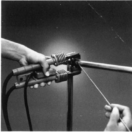
FIG. 18 Electric Resistance Hand Tools Suitable for Soldering Copper Tube
