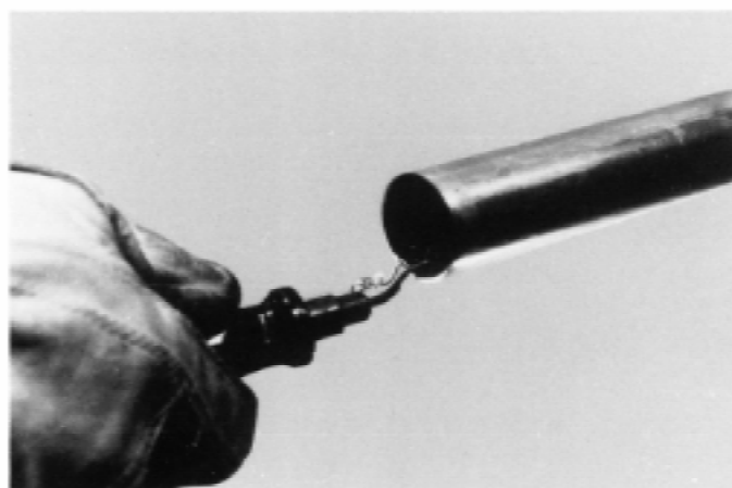
FIG. 5 Reaming: Deburring Tool
