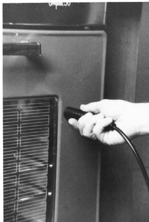
FIG. 4 Applying the Thermesthesiometer to a Vertical Surface
