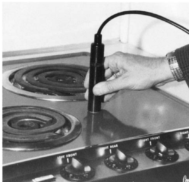
FIG. 3 Applying the Thermesthesiometer to a Horizontal Surface
