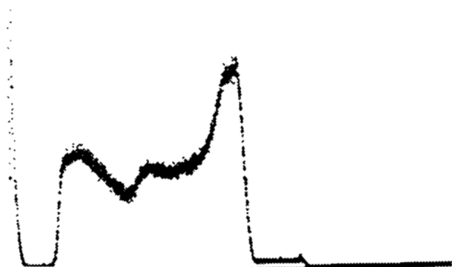
FIG. 8 The ^{252}\text{Cf} Neutron Spectrum Detected by a Moderated ^3\text{He} Proportional Counter and Viewed with a Multi-Channel Analyzer
