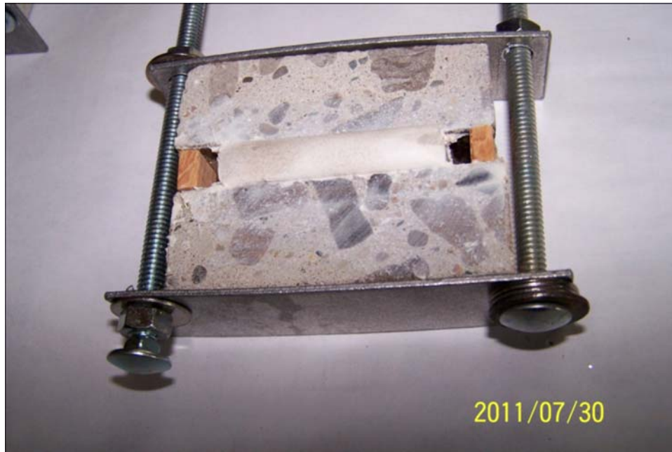
FIG. 3 Clamping Device Holding the Specimen in Compression
