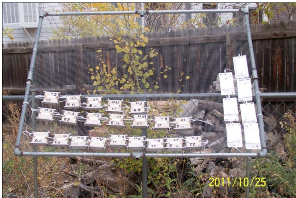
FIG. 5 Specimens Attached to Test Rack
