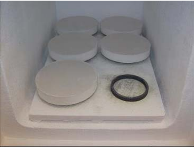
FIG. 6 Specimens Arranged on Hearth Plate Inside Furnace Prior to Testing
