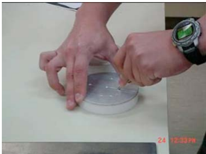
FIG. 9 Sample Preparation—Scoring of Specimen Disk
