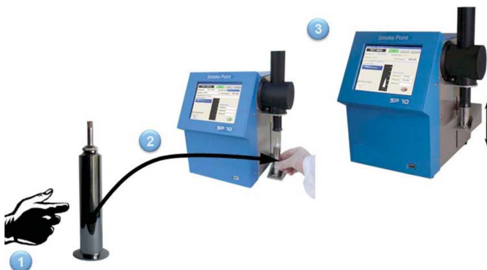
FIG. 8 Candle Positioning with Automated Apparatus
