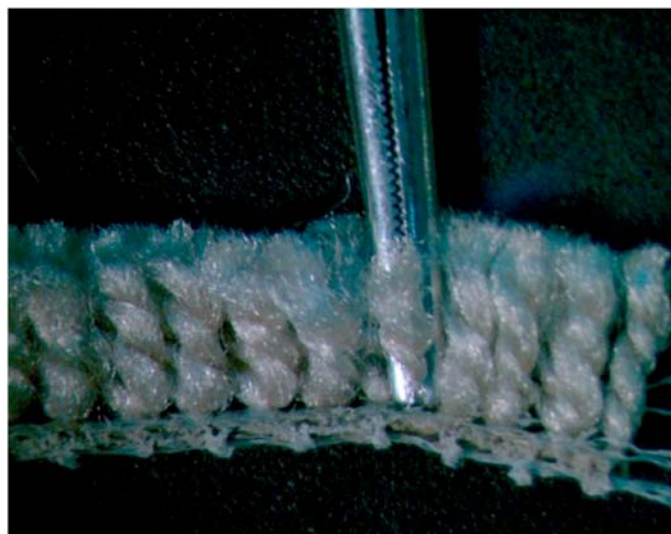
FIG. 3 Tuft Clamp Device Gripping Tuft Leg
