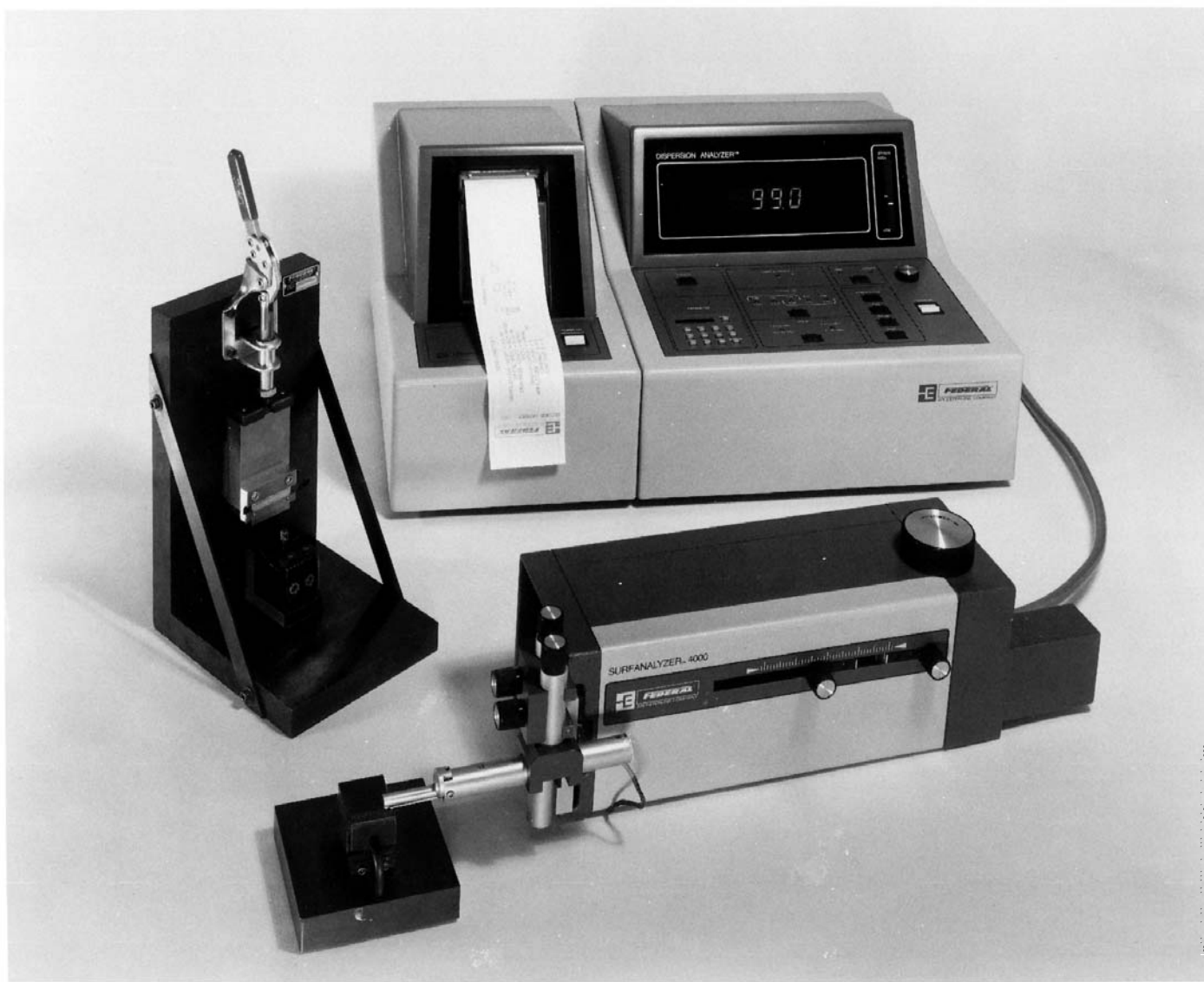
FIG. 5 Components of Profilometer Dispersion Analyzer System
