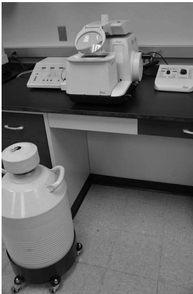
FIG. 2 Rotary Microtome with Cryogenic Attachment for Sectioning Rubber Specimens
