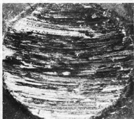
FIG. 5 Typical Test Ball Scars—After Removal
