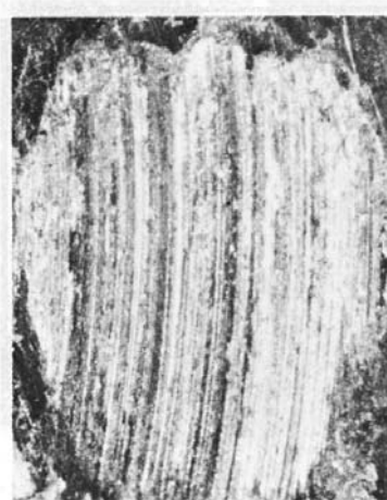
FIG. 7 Typical Test Ball Scars—After Removal
