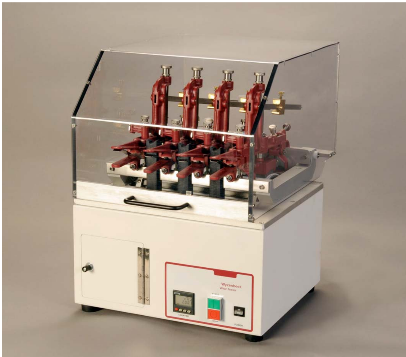
FIG. 1 Oscillatory Cylinder Abrasion Tester
