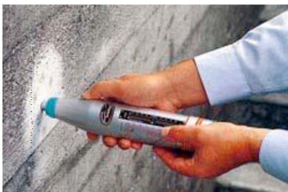
FIG. 3 Example of a Hand-Held Rebound Hammer Perpendicular to the Test Surface in the Field
