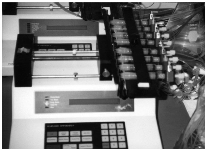
FIG. 3 Photograph of Acid Delivery System
