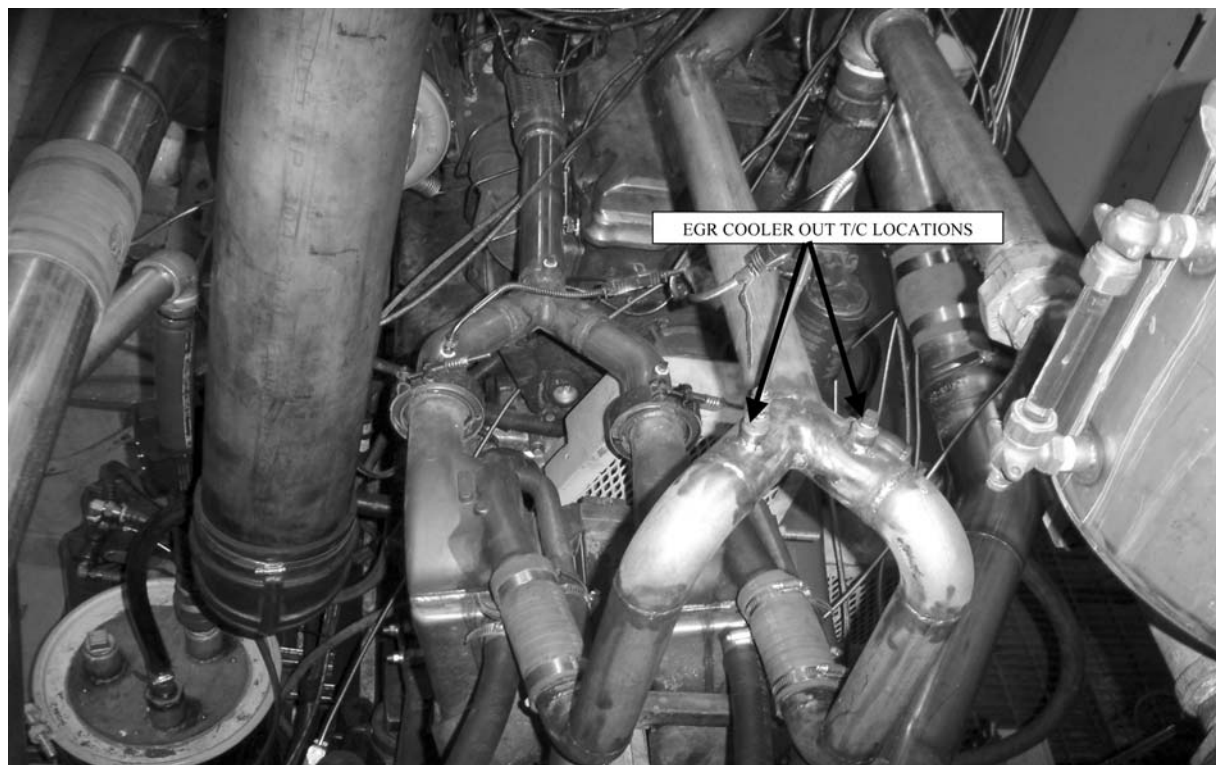
FIG. A1.14 EGR Cooler Out Temperature
