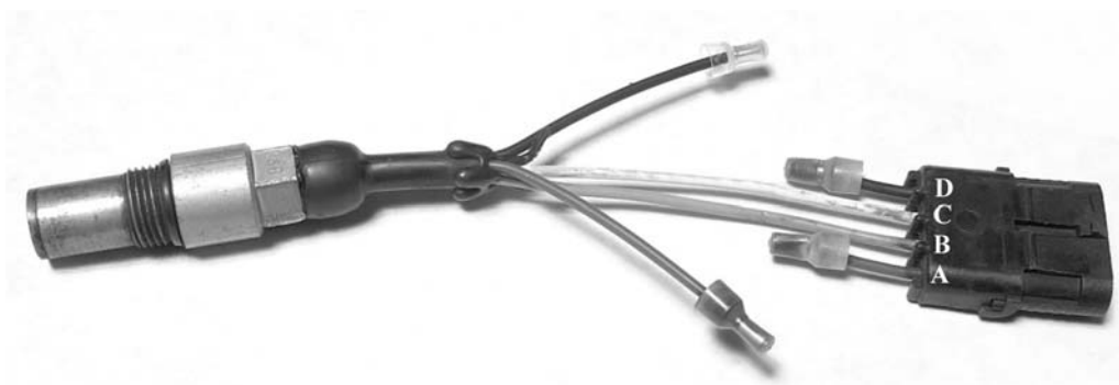
FIG. A4.4 Engine Position Sensor Modifications for ECM 870
