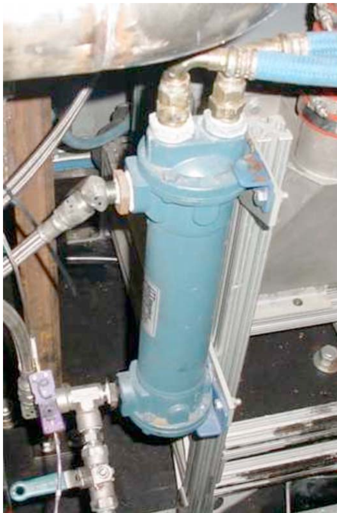
FIG. A4.3 Remote Oil Heat Exchanger
