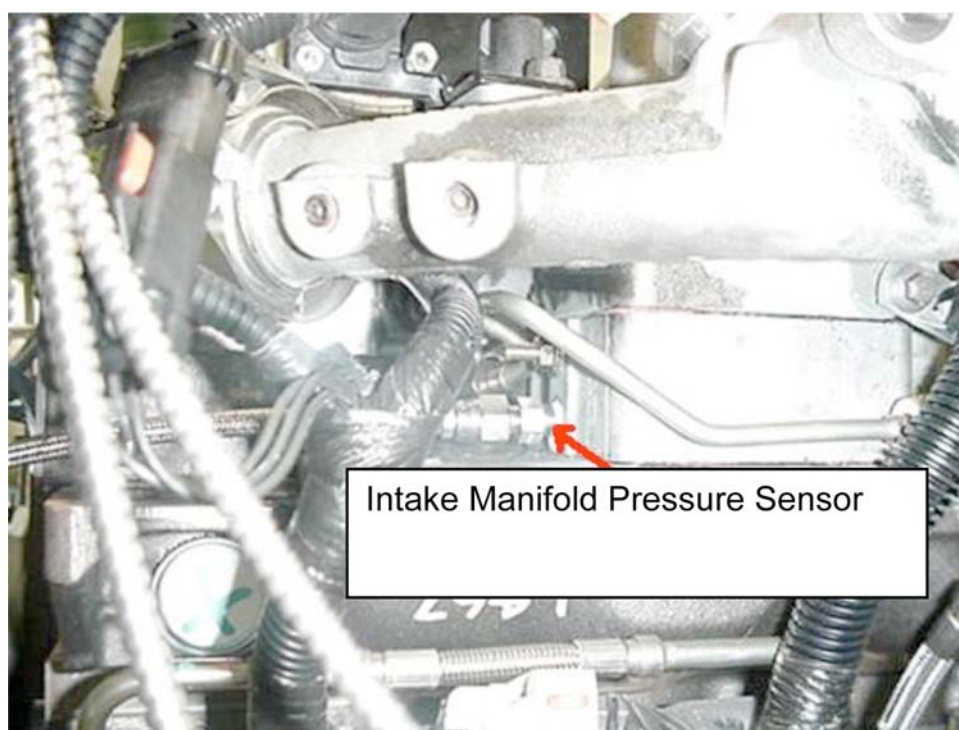
FIG. A4.8 Location of Sensor for Intake Manifold Pressure Measurement
