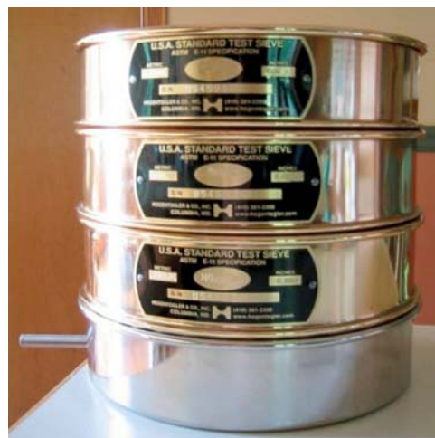
FIG. X1.1 Assemble a Sieve Stack from Top to Bottom as follows: ASTM 19-mm Sieve, ASTM 2-mm Sieve, ASTM 106-μm Sieve, and Collection Pan with Drain Outlet
