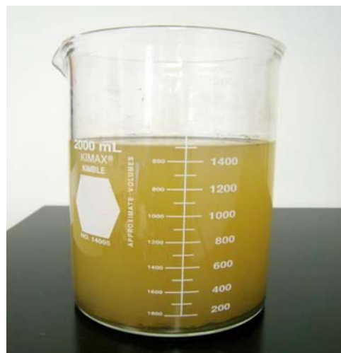
FIG. X1.6 Fine Fraction (<106 µm) that is in Suspension in the 2-L (or Larger) Straight-Walled Container is Covered and Set Aside for at Least 12 h to Allow the Particulate to Settle Out
