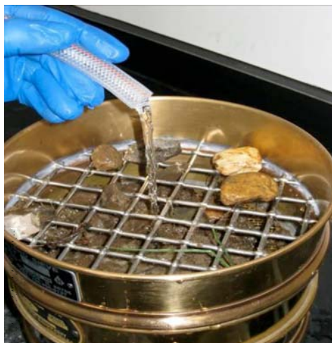
FIG. X1.3 Gently Wash the Coarse Fraction with a Gentle Stream of Particle-Free Deionized Water
