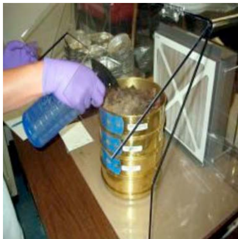
FIG. X1.2 Gently Wet the Sample with a Mist of Particle-Free Water
