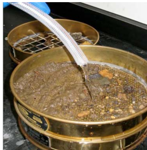
FIG. X1.4 Repeat Steps X1.8 and X1.9 for the >2-mm and >106-µm Fractions
