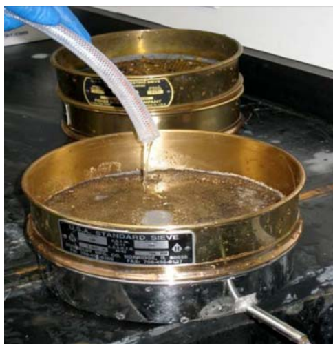
FIG. X1.5 Repeat Steps X1.8 and X1.9 for the >2-mm and >106-µm Fractions
