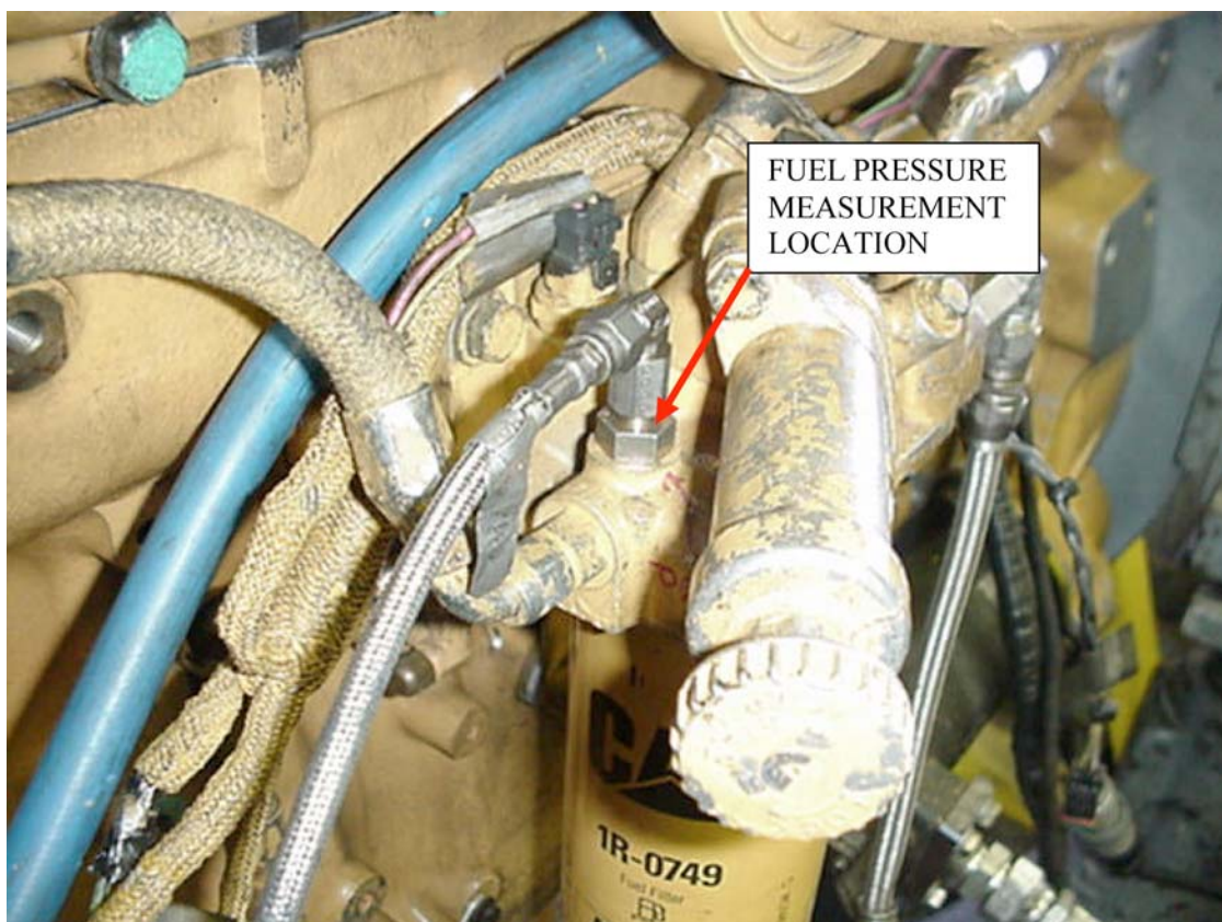
FIG. A4.25 Fuel Pressure Measurement Location
