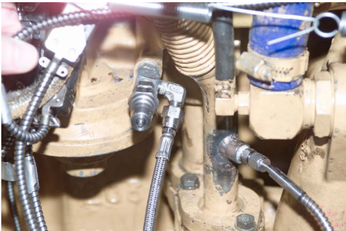
FIG. A4.8 Oil Filter Inlet Pressure Port
