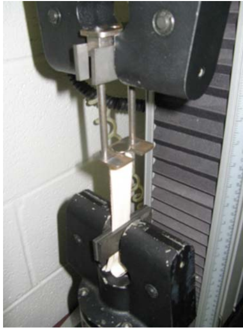
FIG. 5 Specimen Clamping Configuration
