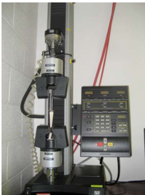
FIG. 3 Tensile Test Machine and Clamped Test Specimen
