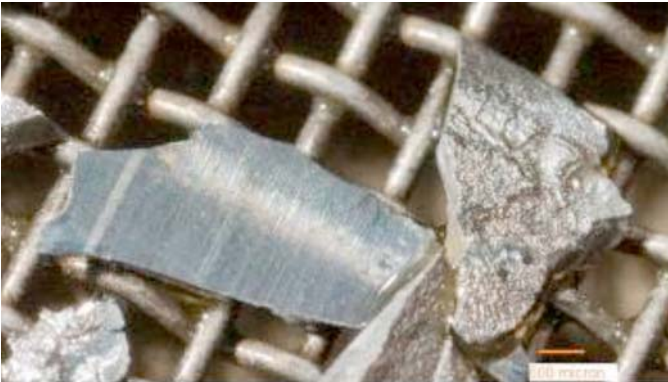
FIG. X3.7 Example of Silver/Gray-Colored Un-Rolled Fatigue Debris
