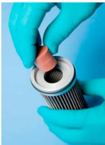
FIG. A1.1 Plug Clean Oil Exit Holes
