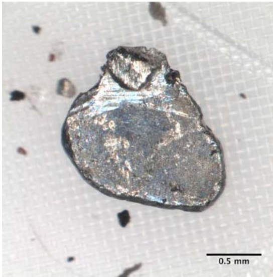
FIG. X3.10 Example of Smooth Edged Debris
