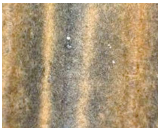
FIG. A2.3 View of Filter Media Showing Valleys Where Debris is Concentrated
