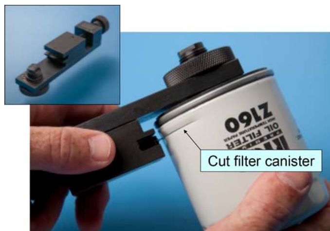
FIG. 1 Example of a Filter Element Cutter
