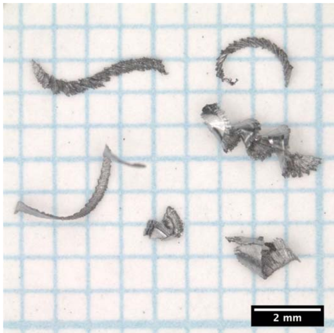
FIG. X3.1 Example of Large Curlicues Indicative of Residual Machining Swarf
