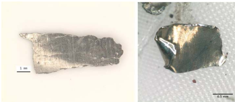
FIG. X3.13 Example of the Smooth Machined Surface of an Un-Rolled Rolling Contact Fatigue Particle (left) and Smooth Plating Particle (right)
