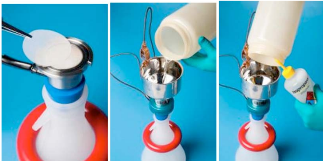
FIG. A1.4 Insert New Filter Patch and Pour Contents into Funnel
