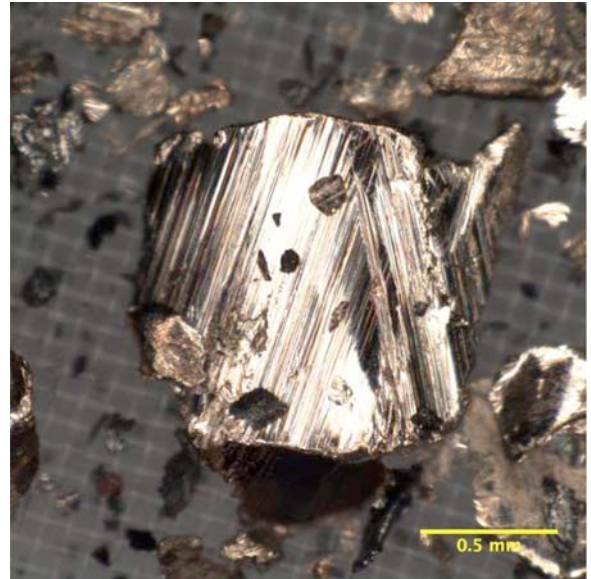
FIG. X3.8 Example of Gold-Colored Debris (Also Showing Adhesive Striations)
