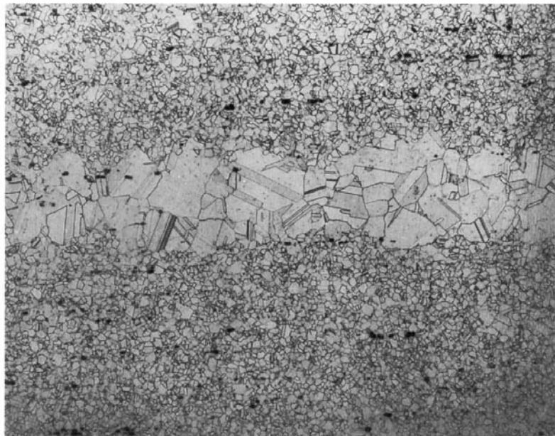
50X Long. Duplex, Banding, 80 % ASTM No. 7, 20 % ASTM No. 2.5
