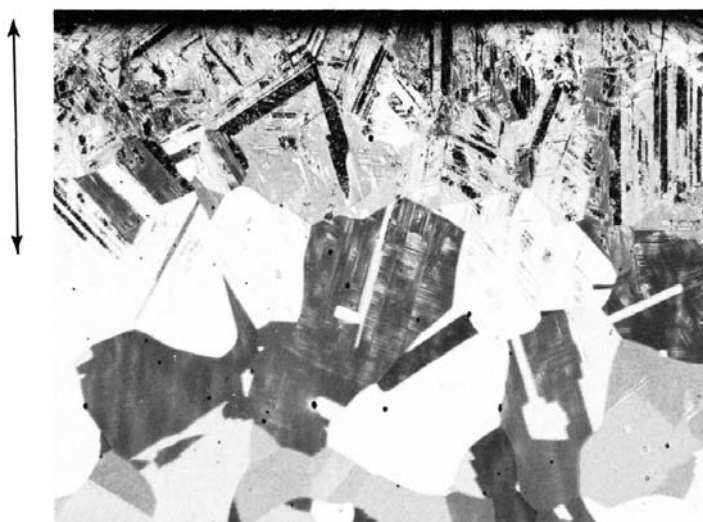
FIG. 10 Example of Epsilon Martensite Formation in the Decarburized Surface Zone of a Solution-Annealed Austenitic Manganese Steel Where the Carbon Content is Less than 0.5 % (100×, Etched With 2 % Nital for 5 s, then 20 % Aqueous Sodium Metabisulphite for 20 s)
