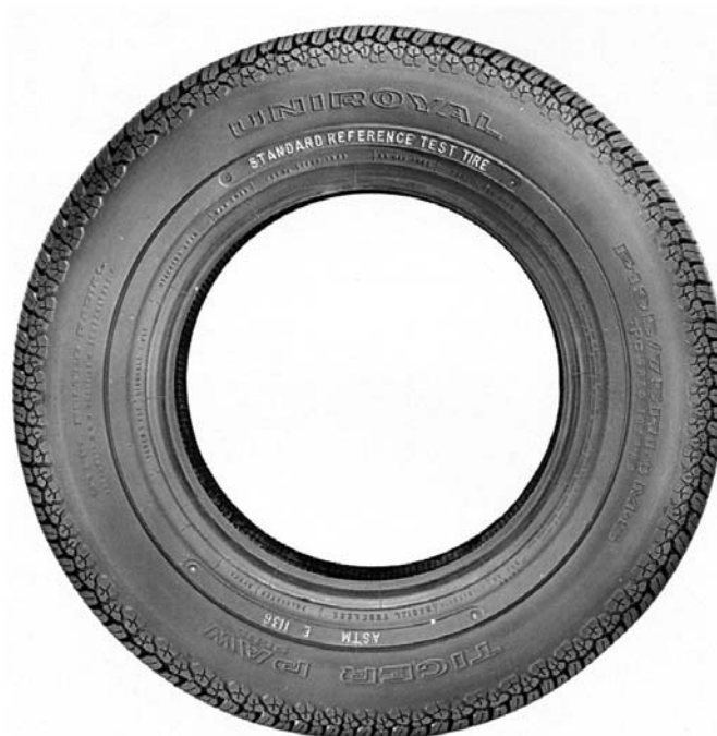
FIG. 2 Side View of the P195/75R14 Radial Standard Reference Test Tire
