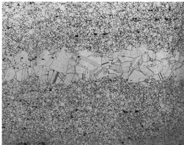
100X Long. Duplex, Banding, 22 % ASTM No. 8, 78 % ASTM No. 3.5
