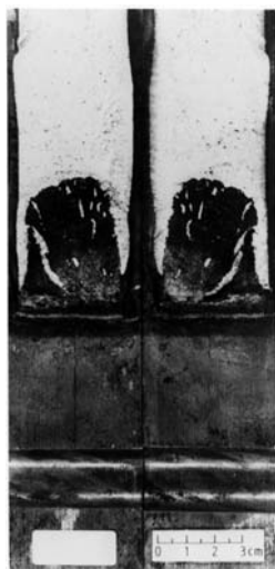
FIG. A1.11 Fracture Surface of a CCA Specimen with an Unacceptably Tunneled Crack Front
