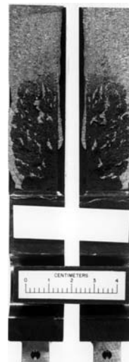
FIG. A1.13 Fracture Surface of a CCA Specimen for Which the Crack has Grown Out of the Midplane of the Specimen but has Remained Mostly Within the Net Specimen Thickness, B_N
