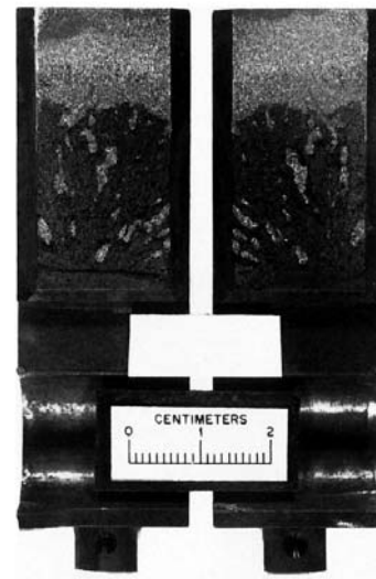
FIG. A1.6 Fracture Surface of a CCA Specimen Showing a Moderate Degree of Ligamentation
