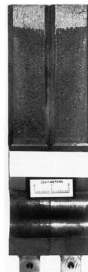
FIG. A1.2 Another Example of an Ideal Fracture Surface of a CCA Specimen
