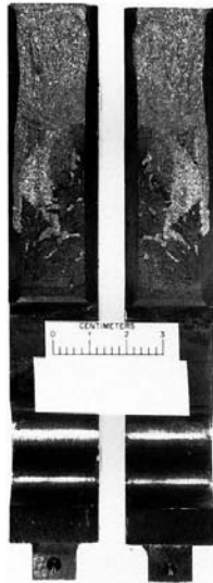
FIG. A1.4 Fracture Surface of a CCA Specimen Showing a Large Remaining Ligament Aligned with the Direction of Crack Propagation
