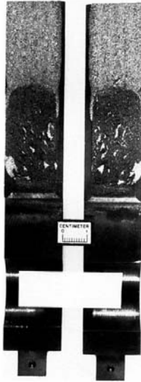
FIG. A1.14 Fracture Surface of a CCA Specimen for Which the Crack has Grown Out of the Midplane of the Specimen and Broken Through the Gross Thickness of the Specimen on One Side
