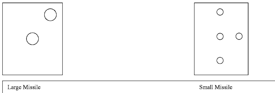
FIG. A4.1 Single Specimen Impact Locations
