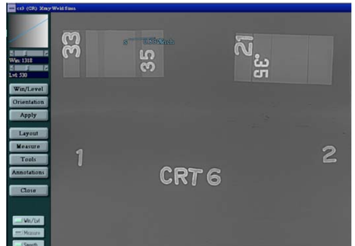
FIG. 25 Wider Window Width (Lower Contrast)
