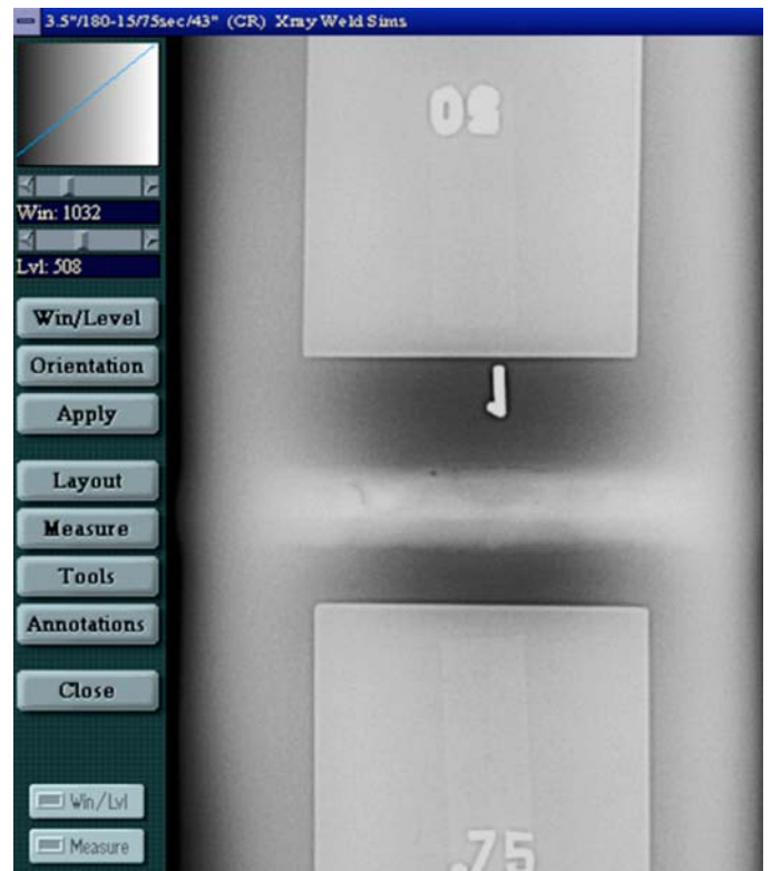
FIG. 26 Pipe Weld Features with Moderate Win-Levels
