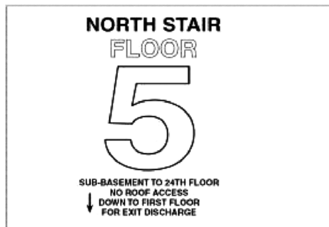
FIG. 11 Stairway Identification Sign
