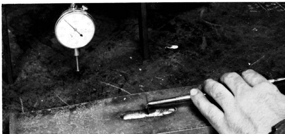
FIG. 7 Methods of Locating the Weld Deposit Properly on the Test Specimen
