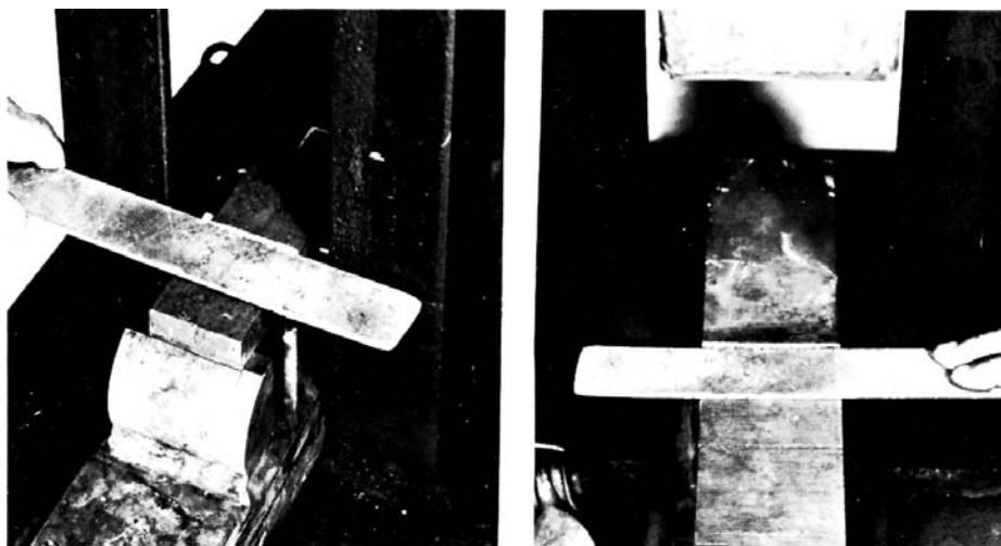
FIG. 12 Method for Alignment of Specimen
